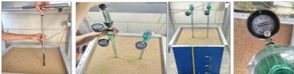
*Plate 7: The stages of installing the Tensiometers and applying vacuum.*
